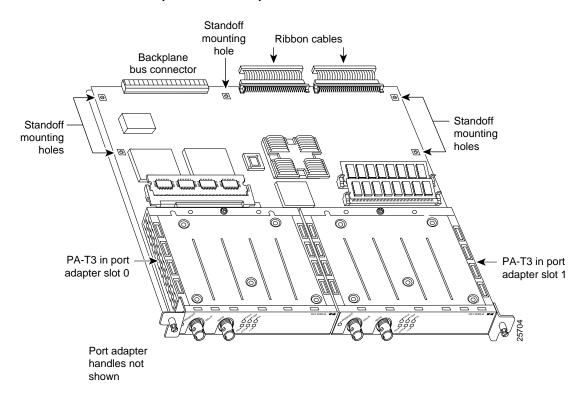
Figure 4-1 Catalyst RSM/VIP2-15 or Catalyst RSM/VIP2-40 with One-Port PA-T3 Serial Port Adapters in Port Adapter Slots 0 and 1
